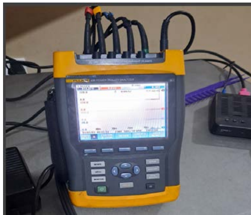
Figure 3.2: Fluke 435 power quality analyzer
