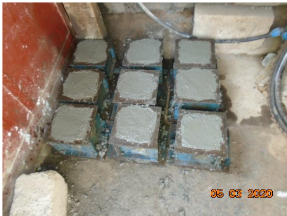
Fig 65; Making concrete tubes for crushing
