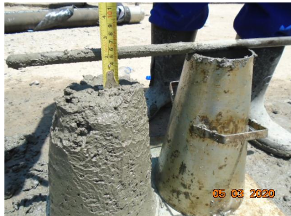
Fig 66; Slump test done on fresh concrete
