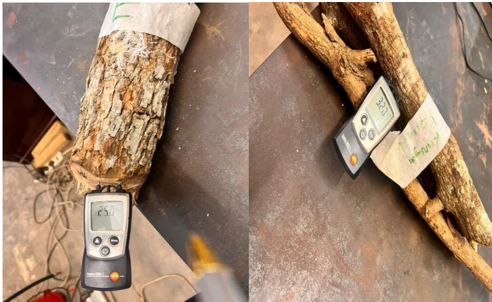
Figure 3.4: Moisture content measured using a moisture meter (Source; Author)
