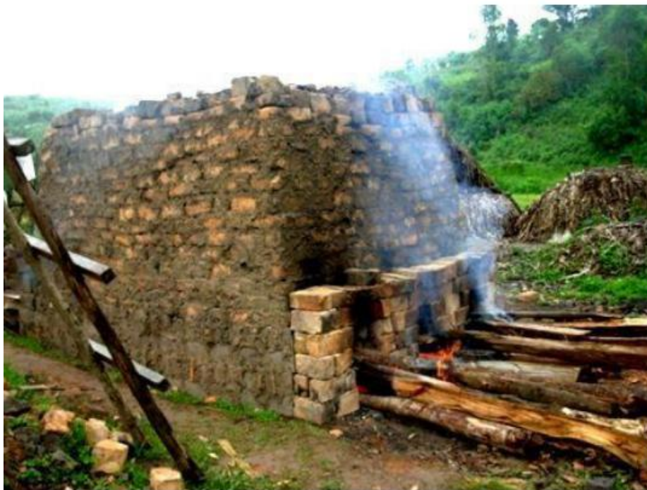
Figure 2.7: Traditional Kiln using firewood (Source; Kayamba & Kwesiga, 2017)
