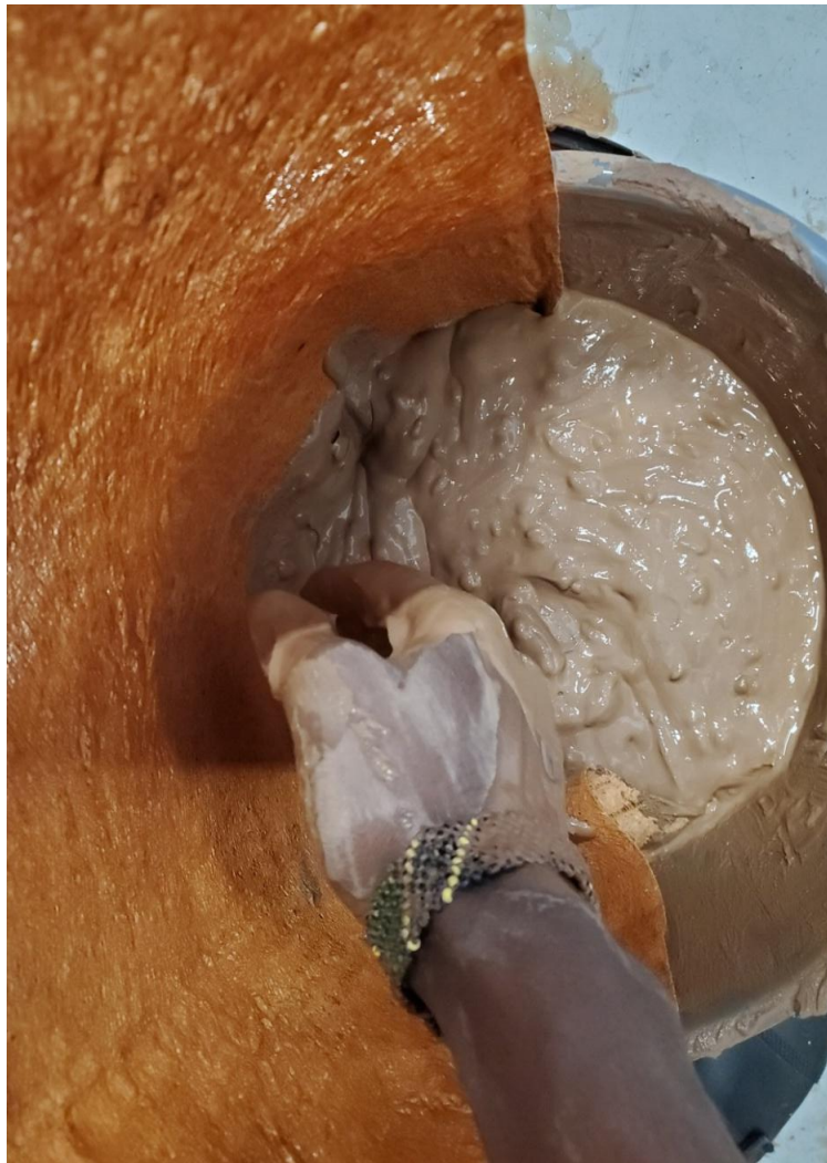
Figure 36: A piece of bark cloth fabric immersed by the researcher in a bucket of clay mixed with water that was later left for one week. Photograph by the Author
