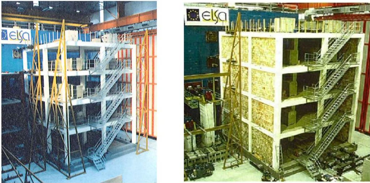
Figure 3.10 Experimental design of frame structure, with and without masonry infill
