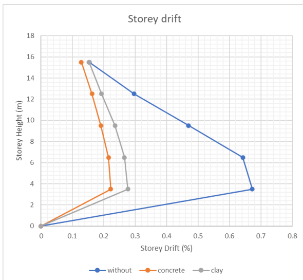
Figure 4.11 G+4 Storey Drift
