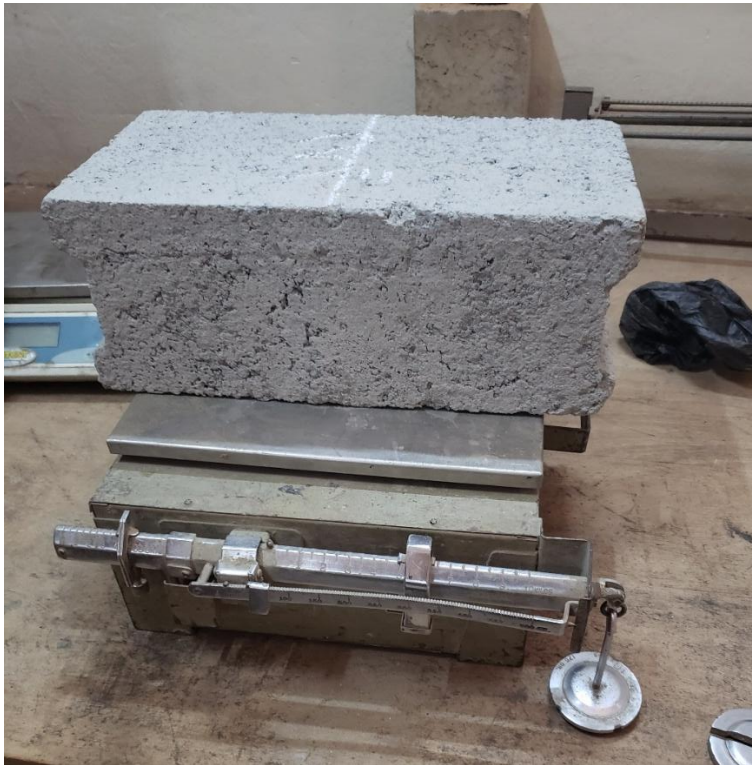
Figure 3.21 Weighing concrete Block sample
