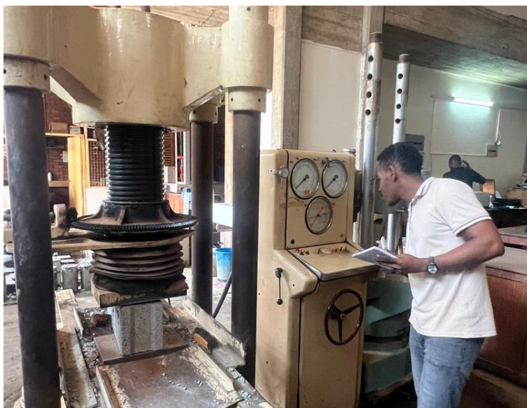
Figure 3.22 Compressive test on concrete Block sample
