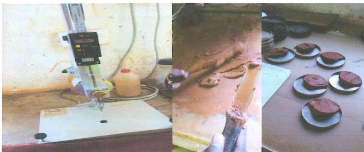
Figure 2:16 The cone penetrometer, paste mixing and samples for moisture content
