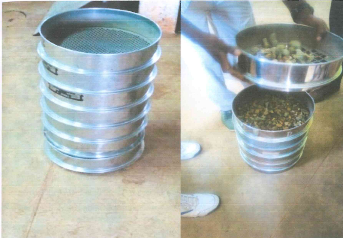
Figure 2:14 Arrangement of sieves and dry sieving during the grading process.
