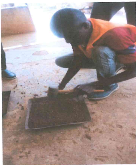
Figure 2:15 Sieving using a 0.425mm sieve
