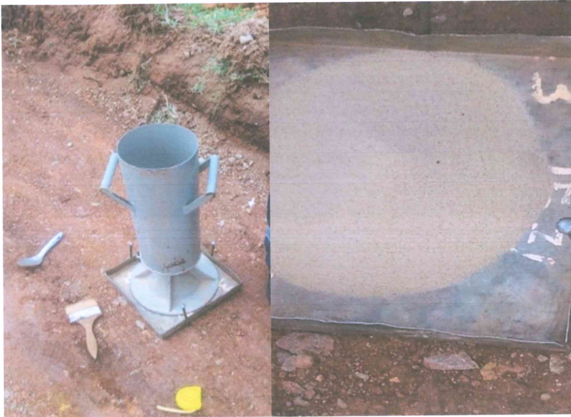
Figure 2:19 Field density test by the sand replacement method
