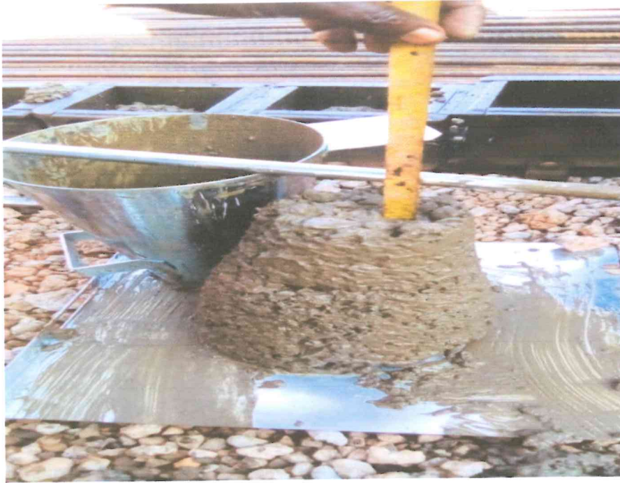
Figure 2:20 Measuring the fall during the slump test
