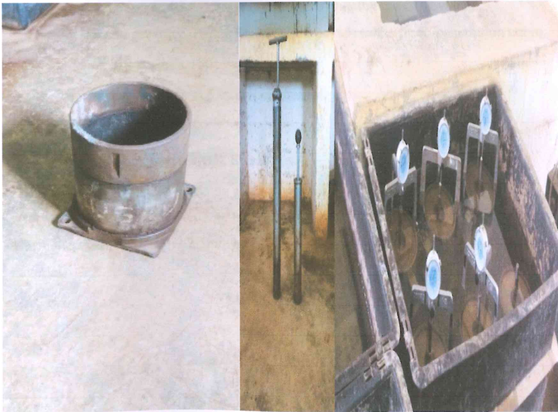
Figure 2:18 CBR moulds, tamping rammers, compacting and soaking of the CBR moulds
