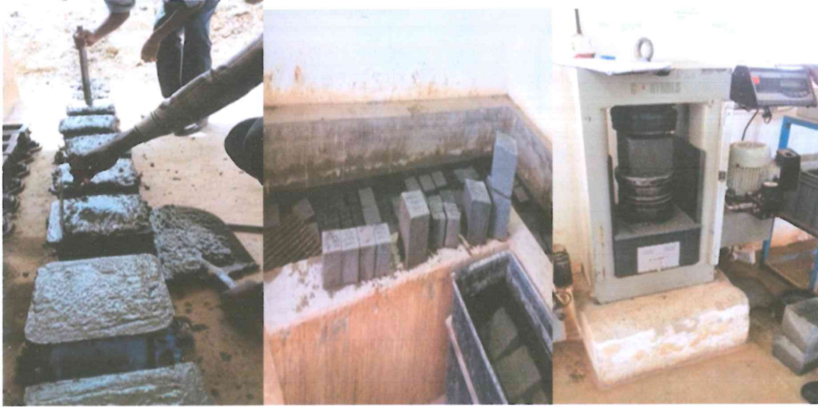
Figure 2:21: Sample compaction in moulds, soaking and compression
