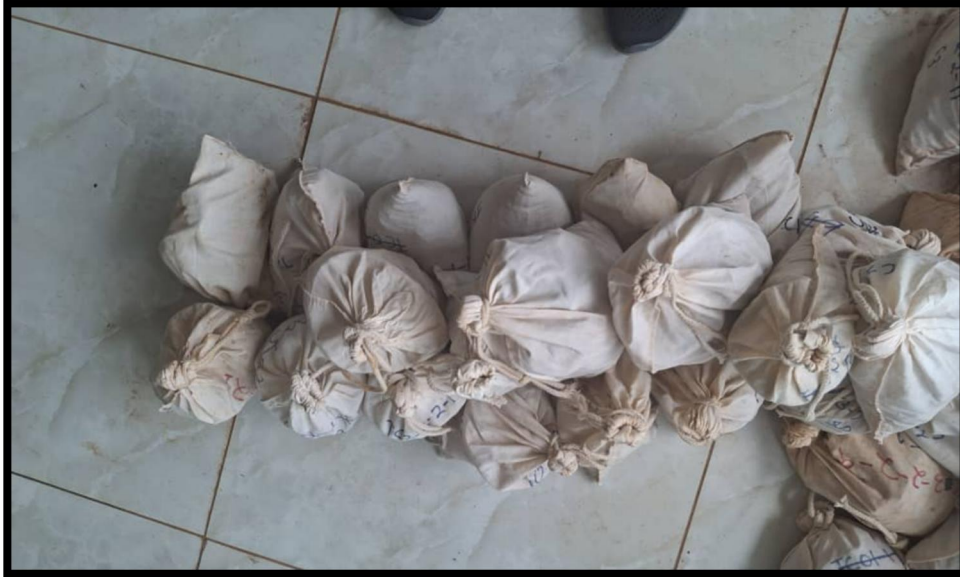
Figure 3.5: showing samples (rock, soil, stream sediments) in well packed material as caution for quality control as the samples were assembled at the Laboratory to undergo sample preparation at mineral dressing lab then after be taken for analysis.
