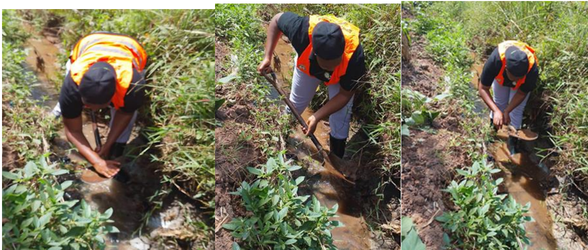
Figure 3.3: Photos showing soil stream sediment sampling in the water channel within the study area. The samples obtained include sediments with clay and silt. This water stream is located in the valley near the mining areas.
