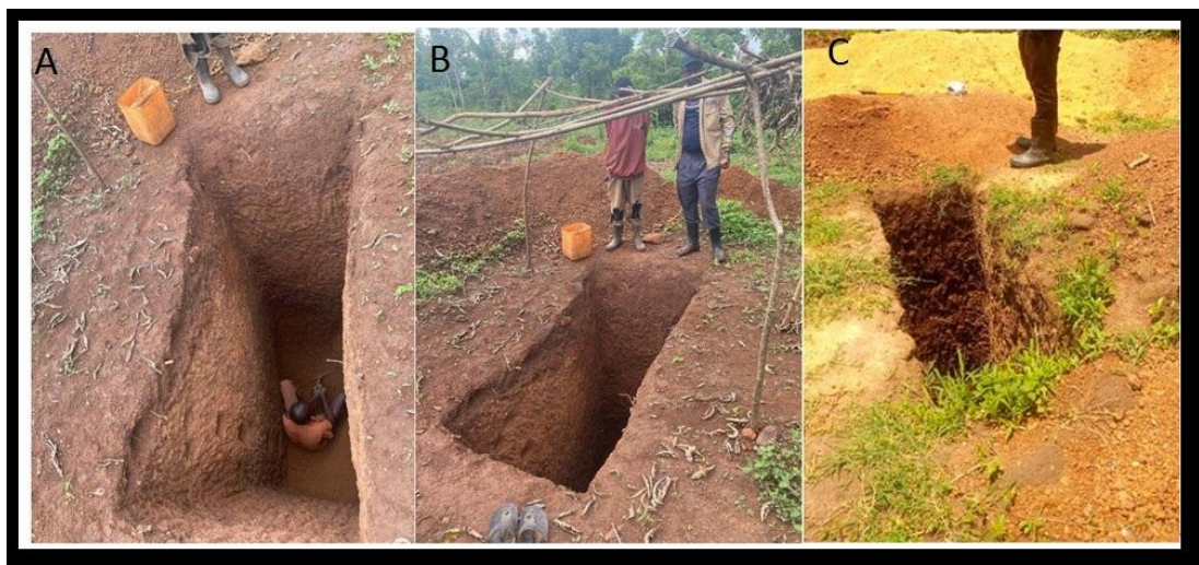
Figure 4.19: Picture showing the mining pits at the site with exposures of different lithology at different soil horizons and the structures within the study area.
