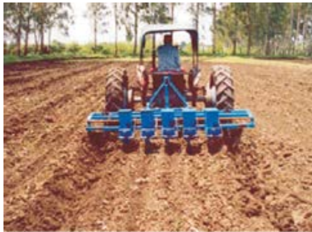
Figure1: Tractor-mounted inclined-plate planter with raised-bed forming attachment for intercrop
