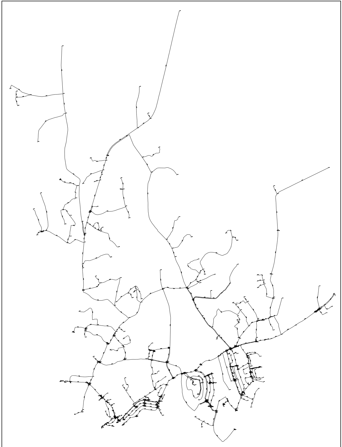
Figure A1-11: Naguru Supply Area Model generated from imported DXF polylines
