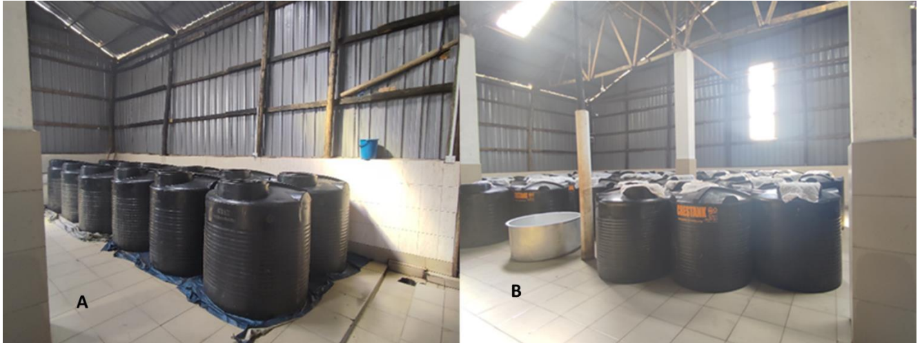
Photo 9: A and B show Kombucha cooling in open drums and fermenting in cover drums at the processing plant
